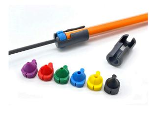
For easy gas- and watertight sealing of cables in miniducts. The miniduct seal is easy to mount on new installations and existing installations. Thanks to the clever design, shifting the seal over the fiber now belongs to the past. Due to the compact design this seal can be installed in every situation, even in locations with difficult access.
